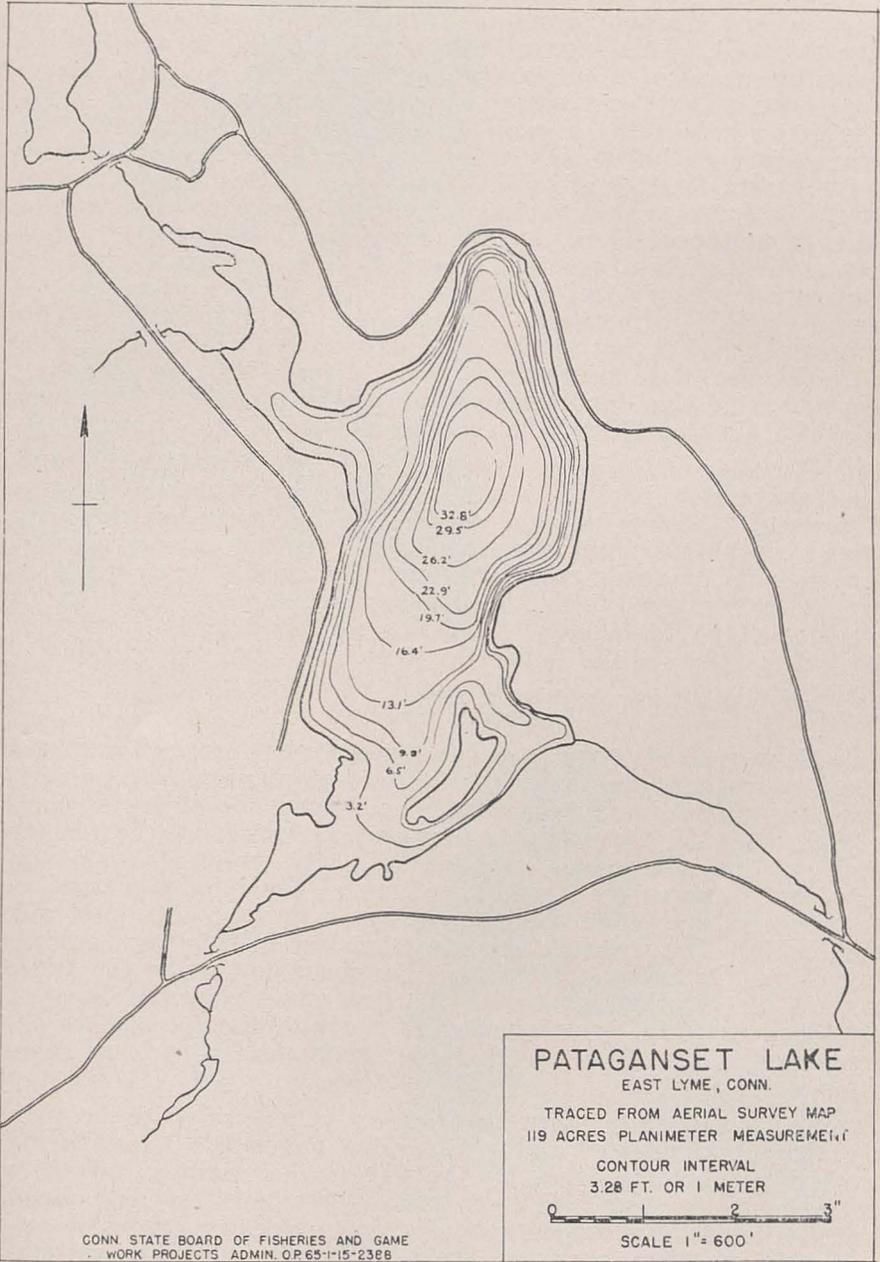
Fig. 9. Example of sounding map made on the larger bodies of water studied by the survey.
