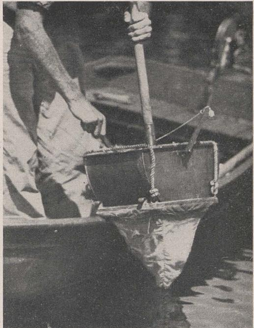
FIG. 13. For sampling in shallow water over sand and gravel bottoms this type of dredge was devised.
