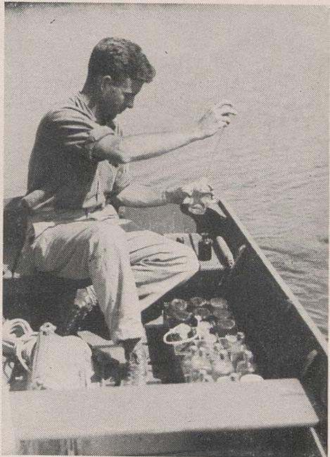
FIG. 11. Preliminary steps in determining oxygen content of water must be carried out in the field.
