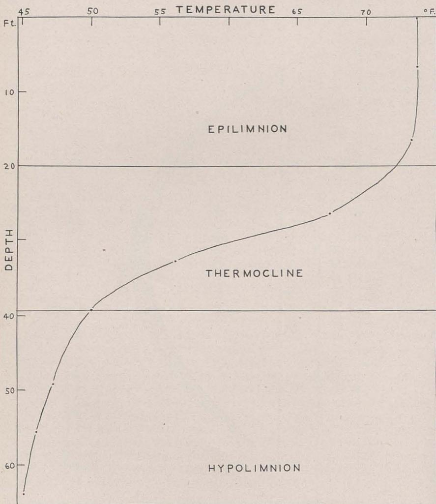
FIG. 4. A typical temperature curve (East Twin Lake, September 1, 1938).
