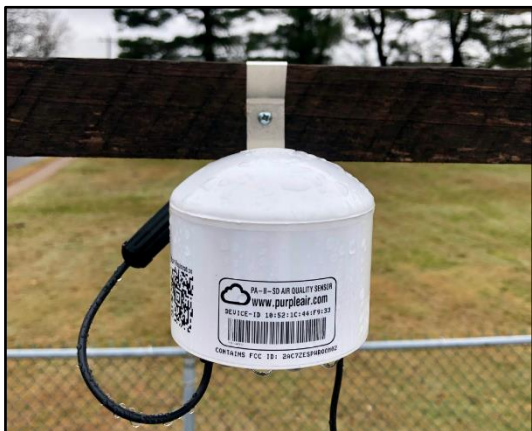
Above: PurpleAir sensor installed at East Hartford monitoring site
