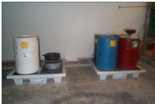
Proper waste storage – closed, labeled drums stored inside with secondary containment
